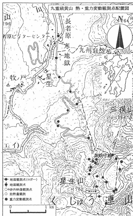
Fig. 3 Observation points of repeat geothermal and gravity measurements in the central part of Kuju volcano after the 1995 eruption. ●: fumarolic and ground temperature by continuous recording, ●: ground temperature, ○: infrared imagery, ○: heat discharge rate, ●: gravity.
