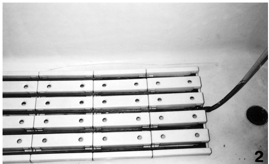
Photo 4-2 : Bubbling system in the bottom of bathtub.
